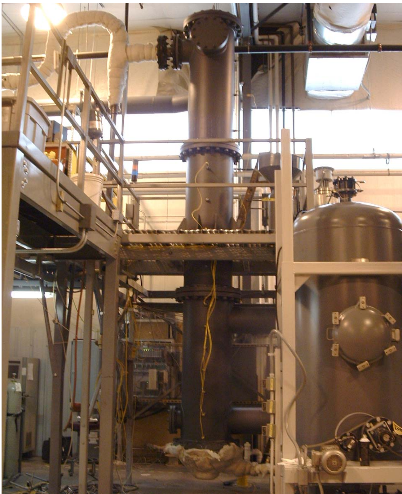
Figure 7: Gasification system shortly after installation (reaction vessel at center of photograph; pressurized fuel hopper at right).
